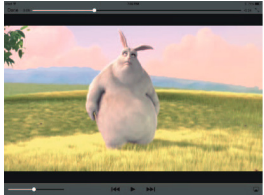
Figure 2. Default controls of a mobile video player as used on the Apple iPad. In the lower part of the screen we can see fast-forward/reverse and play as well as volume control (which, however, can be controlled by other means, e.g., hard buttons, as well). In the upper part of the screen we can see the seeker-bar to be used for navigation by scrubbing. All controls are usually hidden during playback and need to be enabled by a tap gesture.
